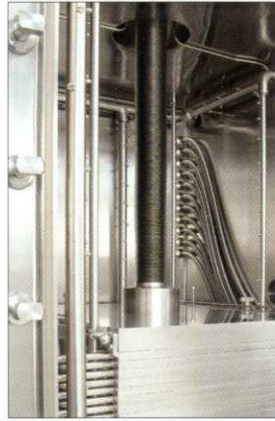
Shelf system with simple adjustment of distance between shelves
