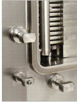
Safe, automatic door bolt used during drying and sterilizing
