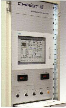
PLC system interface with SCADA software LPC 32 (FDA approved)
